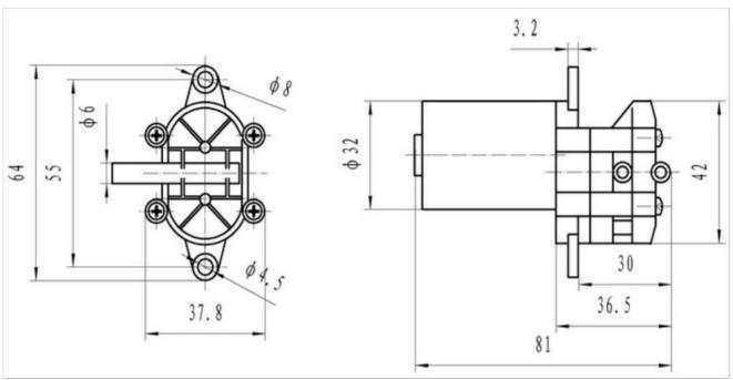
TG-02S size (note: TG-02B with the same pump head size, just motor with length of 104mm, width of 38mm)
